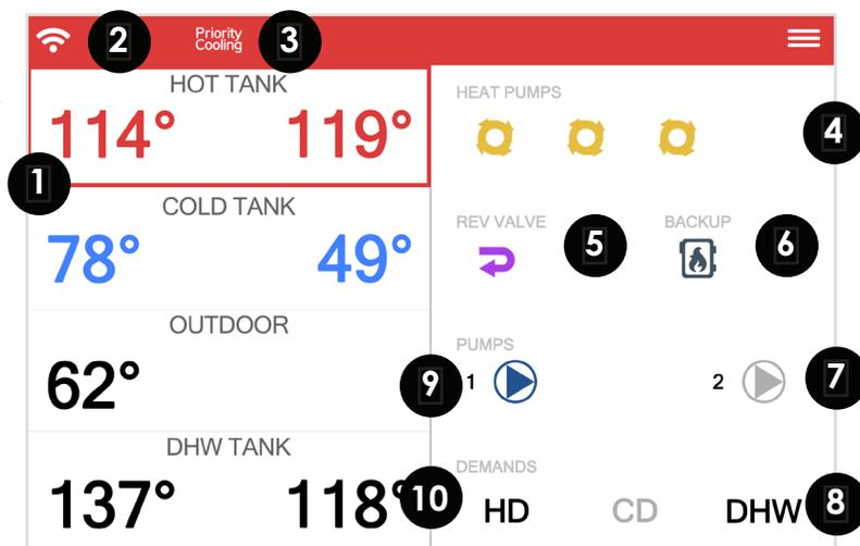
Accessing the menu of the ECO-0600 is done by pressing the menu button (3 lines) in the top right corner.
