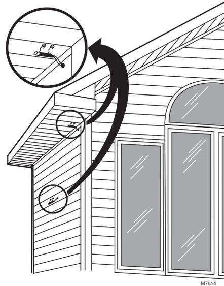
**Fig. 27. Typical locations for C7089U1006 Outdoor Sensor.**
