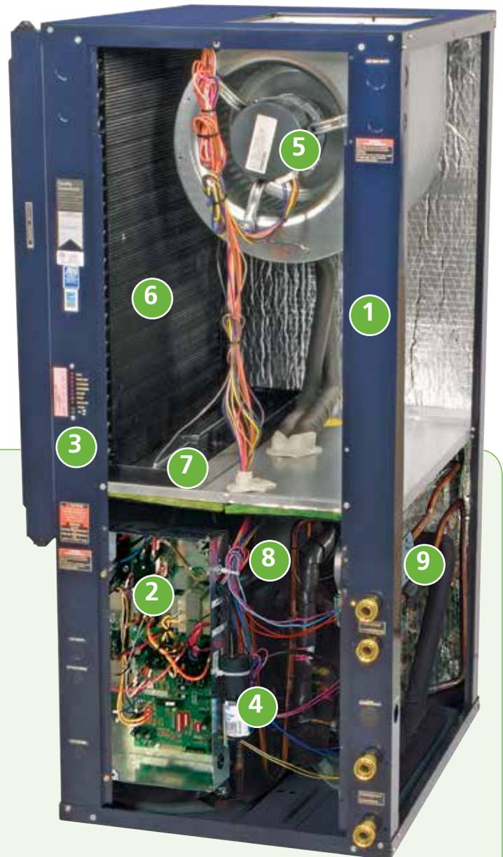
**7 DRAIN PAN** The plastic, corrosion-proof drain pan resists bacterial growth and eliminates the possibility of condensate flooding through the use of electronic overflow protection.
