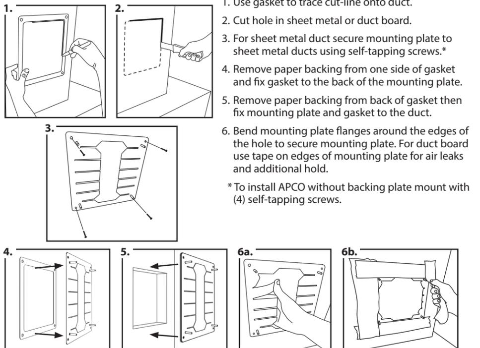
\*To install APCO without backing plate mount with (4) self-tapping screws.
