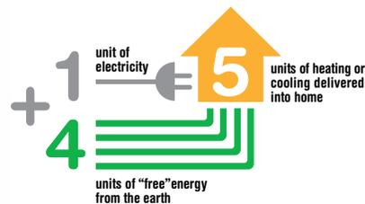
dollars worth of energy output to heat and cool your home, representing an efficiency rating of nearly 500%! Compare that with conventional furnaces that deliver less than 97 cents worth of energy for the same dollar.
